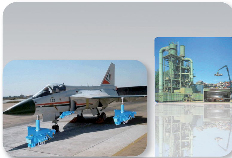
Bearing unit for a GVT Ground Vibration Test for aircraft & an air spring bearing for an industrial shredder
